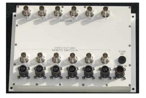
The VSA-103 is a Six Camera In, Six Monitor Position Out Video Switcher. Each of six output positions can select any of the input cameras by the use of a six position Rotary Selector Switch. The system is operated with nominal 28 VDC input power. Input and output impedance is 75 ohms with Unity Gain.
