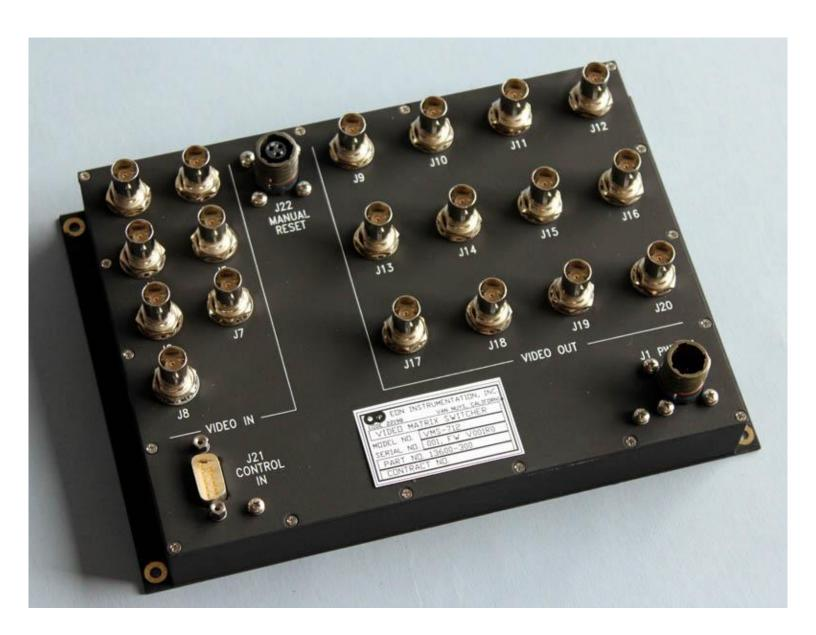
The HD-SDI Video Matrix Switcher is EON Instrumentation's brand new high-speed digital video product. The VMS-712 provides video switching and distribution support for high-definition digital video interfaces.
