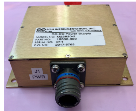
The M-141300-1 300 Watt power supply (left) and M-22820-2 20W power supply (right)
