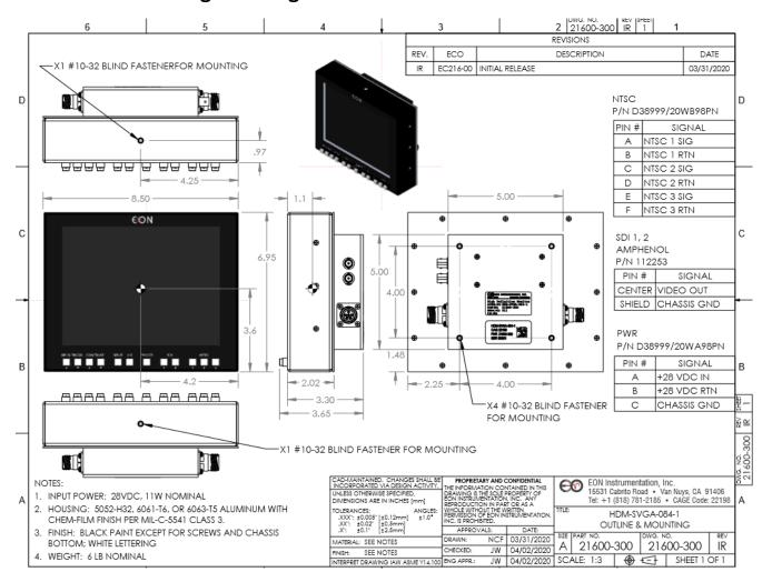
Power mating connector: 26WA98SN NTSC Signal mating connector: 26WB98SN SDI Signal mating connector: Any BNC plug
