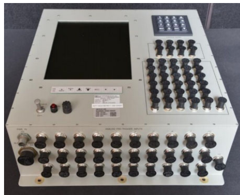
PCAB Blanker for the Aegis weapon system
